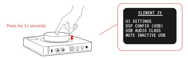
Pressing down on the Volume Knob for 3+ seconds enters the Options Menu. Turn the knob to navigate up/down the Options menu. Push the knob to make a selection.
